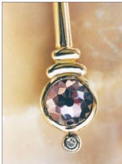
Figure 13 – Purple gold used in a pin. The purple colour is given by the AuAl 2 intermetallic compound.
